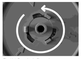
Fig. 4.2.4: Removing the filter retainer
