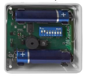
Fig. 3.5.1: Coding switch for coding
